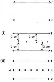
From the final figure obtained, the required locus is the line AB which is parallel to both the given lines l and s and is also equidistant from both the lines.
