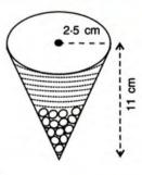
Vol. of lead shots dropped = Vol. of water that overflows
